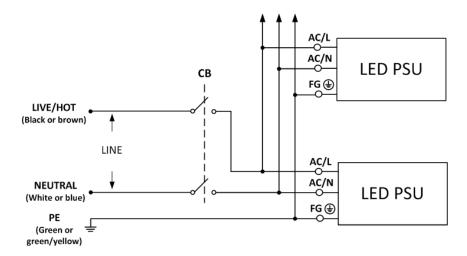
(6) The maximum number of NPF-40-20 that can be connected to a circuit breaker at ~230V(AC) is shown as below.
